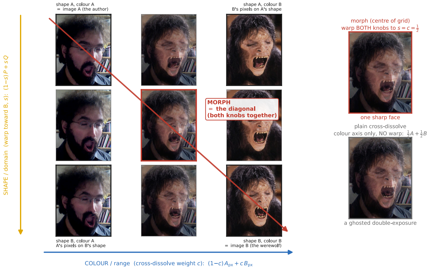
Figure 11.3.2 (reproduced). The two knobs of a morph, as orthogonal axes. One axis, range (color): the cross-dissolve C(x) = (1 - t)C_0(x) + tC_1(x) , a linear blend of pixel values. Other axis, domain (shape): a feature point interpolated as a vector, V = (1 - t)P + tQ , sliding the feature's location from where I_0 puts it to where I_1 puts it. A plain cross-dissolve moves along the color axis only (ghosts); a true morph is the product: interpolate position and color together. The corners of the square label the four extreme combinations.
