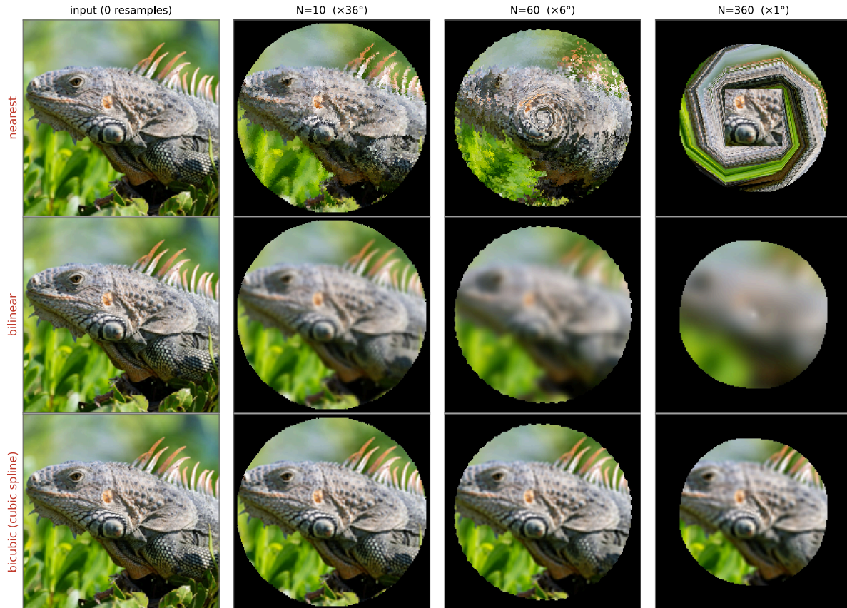
Figure 6.5.15 (reproduced). Andrew Adams' rotation challenge, and how much the resampling filter matters. Each image is rotated a full 360^\circ in N = 10, 60 , or 360 equal steps, every step resampling the previous result; it is the same total rotation, just chopped into more or fewer passes, so more (smaller) steps compound more damage. The three rows repeat the experiment with a different resampling filter: nearest-neighbor, bilinear, and bicubic (cubic spline). Nearest jitters and loses registration; bilinear (a mild low-pass) washes the iguana's fine scales into mush by N = 360 ; bicubic, whose negative lobes restore some of the contrast each pass would otherwise lose, holds the detail markedly longer. A validity mask blacks out the corners that ever rotate out of frame, so the kept region shrinks toward the inscribed disc. The lesson: the resampling kernel is not a detail: it is the difference between a tool you can trust and one that quietly destroys your image.
