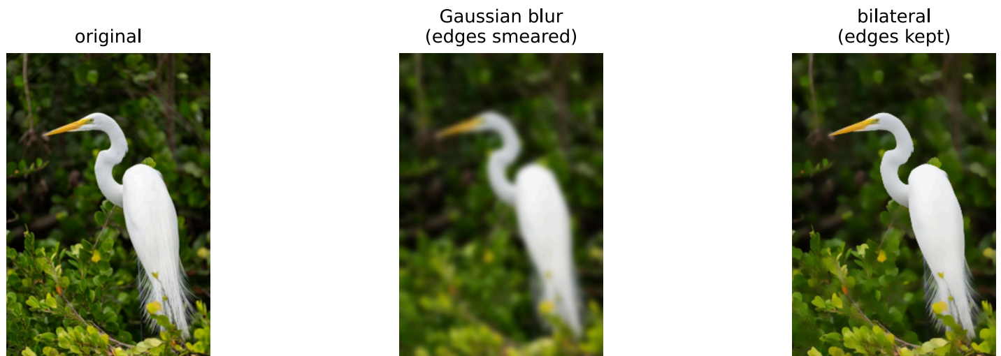
Figure 10.1.2 ( reproduced ). The bilateral filter on a real photograph. Left, the input: a white egret against busy foliage. Center, a plain Gaussian blur of the same radius: it smooths the foliage texture but also smears the bird's edges into the background. Right, the bilateral filter: texture and noise are smoothed away within each region while the strong edges, the bird's silhouette and the beak, stay crisp. The same behavior as the 1-D scanline, now on a 2-D image.
