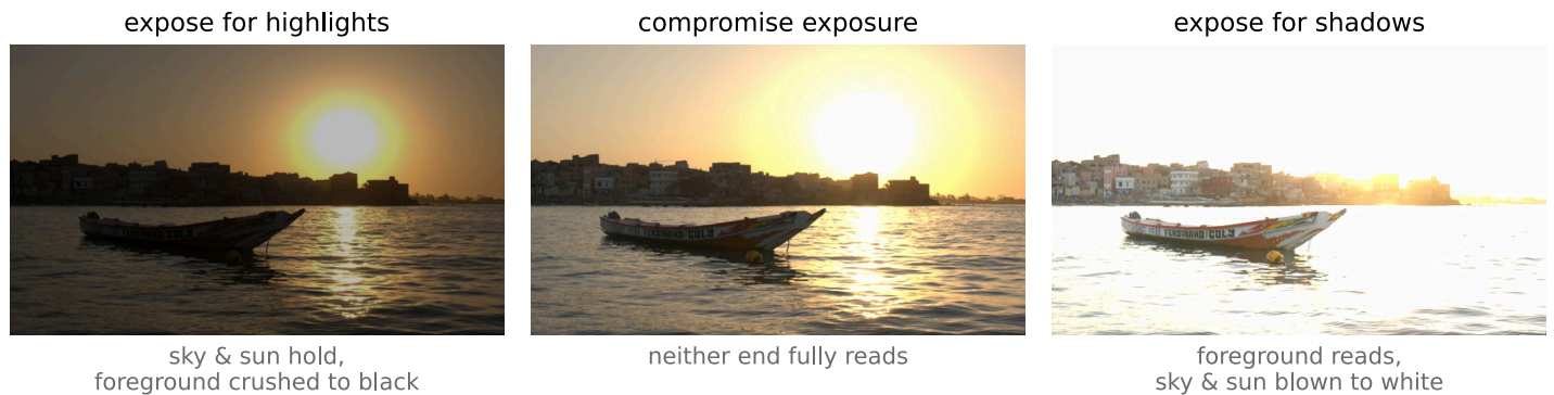
Figure 2.8.14 (reproduced). The dynamic-range problem. One high-contrast scene (a sunset over water) developed at three exposures: expose for the highlights and the foreground is crushed to black; expose for the shadows and the sky blows out to white; the compromise loses both ends. No single exposure holds the full range: the motivation for high-dynamic-range merging of multiple exposures.
