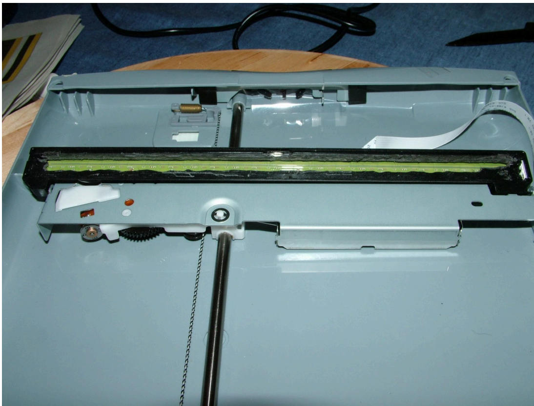
Figure 4.6.2 ( reproduced ). A scanner's linear sensor bar. The contact-image-sensor (CIS) bar of a flatbed scanner reads one line of the page at a time; the carriage sweeps it down the page, spending time to build the second (vertical) spatial dimension a one-dimensional sensor lacks, and color comes from three RGB-lit passes or a tri-linear sensor with three colored rows. The purest everyday example of trading a scene axis for the measurements the hardware cannot make at once. (Photo: Michele M. F. / Latente, CC BY-SA 2.0, via Wikimedia Commons.)
