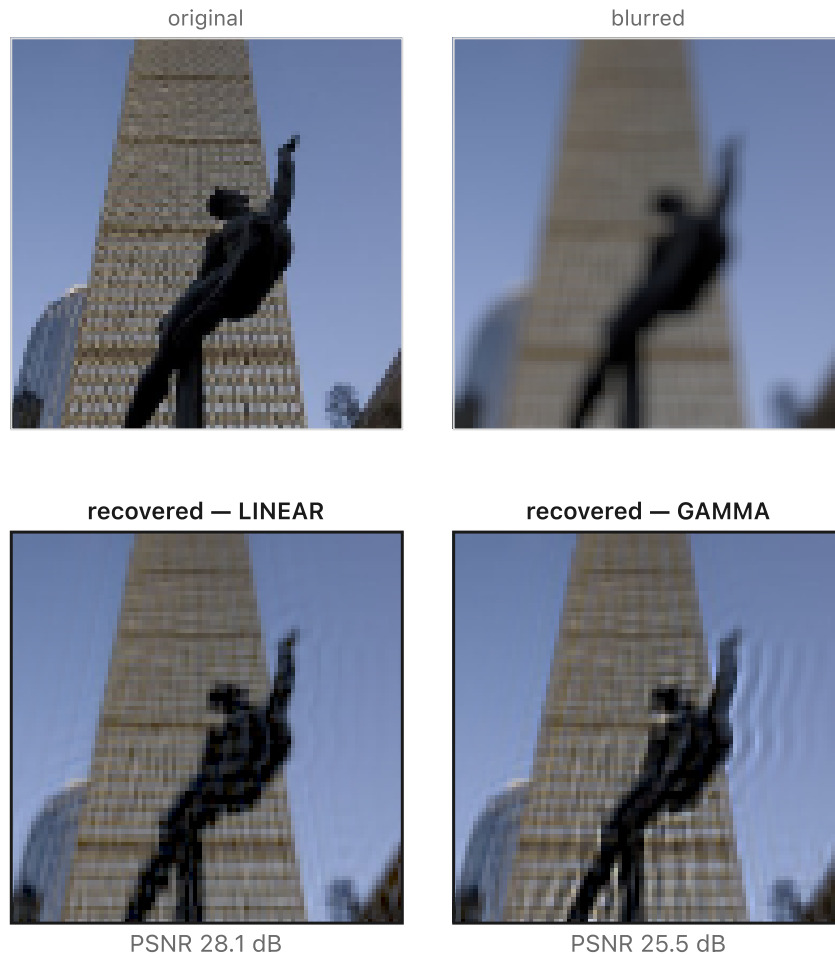
Figure 6.8.1 (reproduced). Deconvolution in linear vs gamma-encoded values. A sharp source (a real photo, Prudential by default, or a high-frequency grating dipping into the shadows, whose contrast and period you set) is blurred in linear light (box or Gaussian), then the blur is inverted two ways. Recovered (LINEAR): 220 Landweber iterations on the linear values, which fits the physical model. Recovered (GAMMA): the same iterations on the gamma-encoded blurred values, as if codes were light, which is the wrong model because gamma and blur do not commute (halos, lost contrast). Neither recovers the source exactly, since the iterations are finite and the blur removed information. The PSNR under each panel quantifies the gap: at the default settings 28.9 dB for linear against 26.0 dB for gamma, an ordering that can change with the source and the blur. The gamma error particularly affects the photo numerically, yet is not always visually obvious: most local neighborhoods are nearly constant, so locally linear: it is the grating that shows it plainly.
