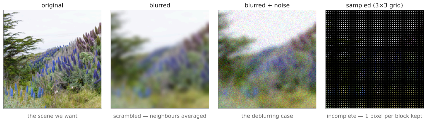
Figure 6.1.1 (reproduced). The same scene, reaching us imperfect in three different ways. From one photograph: blurred (the information scrambled, since a blur averages neighboring pixels together), blurred with a little sensor noise on top (the deblurring case of the sections that follow), and sampled on a coarse grid (incomplete: only the center pixel of each 3 \times 3 block survives, the rest dropped). Each is a different way the forward map discards or corrupts information, and each needs a different inverse to undo it.
