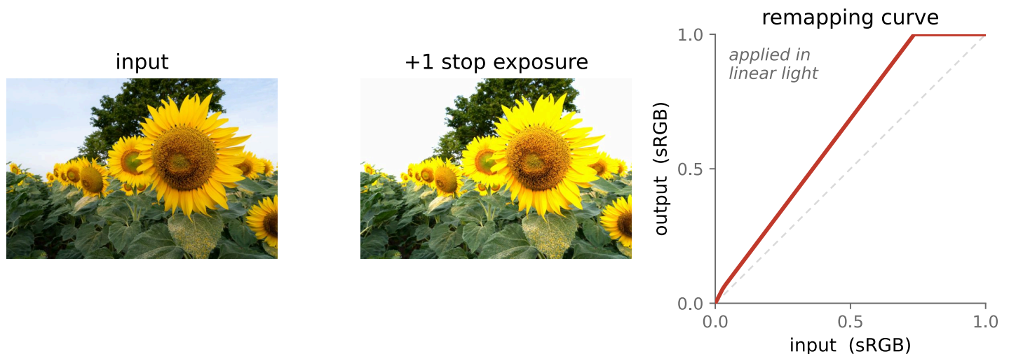
Figure 8.3.2 (reproduced). Exposure as a multiply in linear light. Left, the input. Center, the same photo at +1 stop ( \times 2 in linear light), brighter throughout, with the brightest highlights clipped to white. Right, the transfer curve L_{\text{out}} = 2^s L_{\text{in}} drawn in display (sRGB) space: it bows above the 45^\circ diagonal, lifting the shadows strongly and flattening into the ceiling at 1. The 45^\circ diagonal (no change) is shown for reference.
