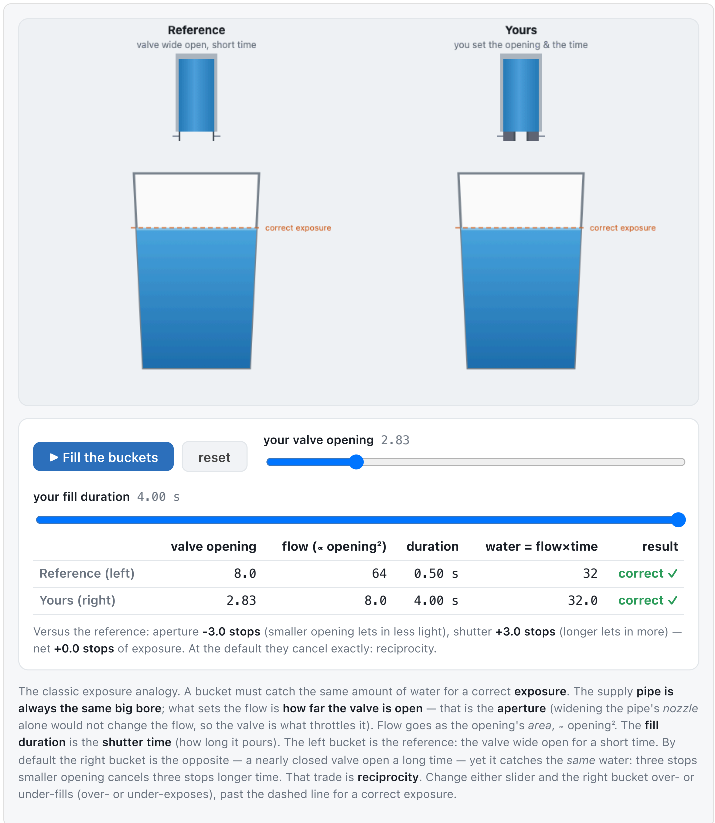
Figure 5.2.1 (reproduced). Interactive: the faucet-and-bucket exposure analogy. Two buckets fill from faucets; the water caught is the exposure and the dashed line marks a correct one. The faucet diameter is the aperture (flow rate follows the opening's area, \propto \text{Ø}^2 ) and the fill duration is the shutter time. The left bucket is a fixed reference (wide faucet, short time); the right one you control, defaulting to the opposite (a narrow faucet open a long time), yet it catches the same water, because three stops of smaller aperture cancel three stops of longer time. Press to fill the
