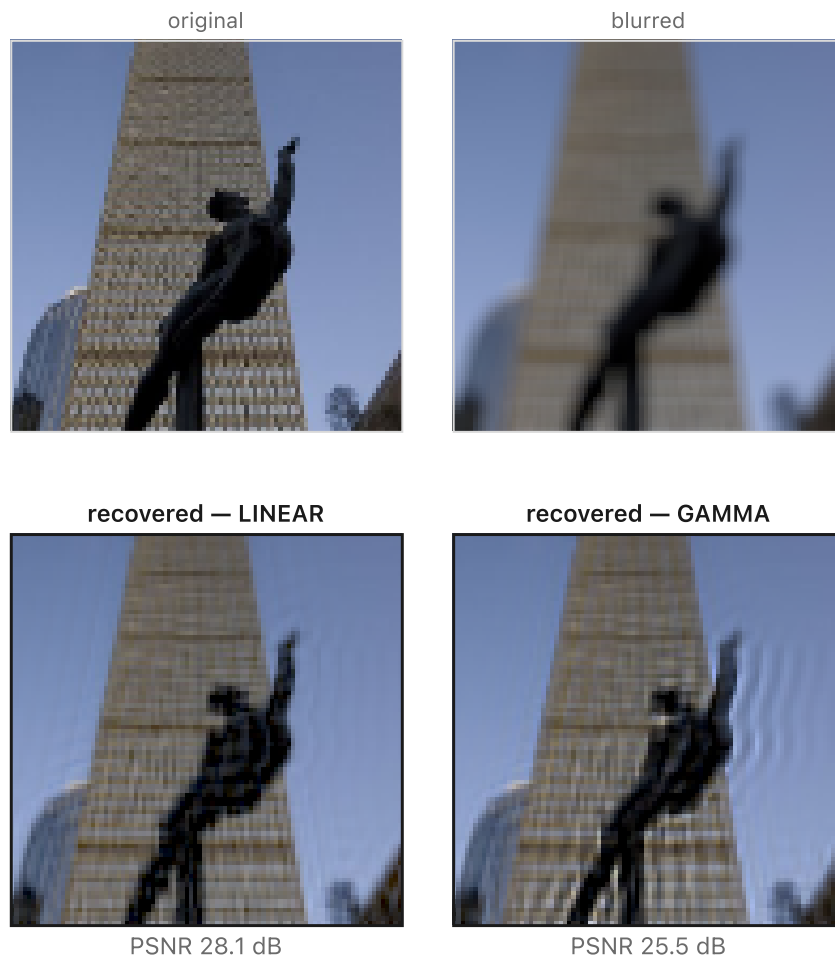
Figure 6.8.1 (reproduced). Deblurring belongs in linear light. A sharp image is blurred in linear light (a true average of light), then the blur is inverted two ways: on the linear values (the right model) and on the gamma-encoded values (the wrong model, with halos and lost contrast, because gamma and blur do not commute). Both use the same finite number of iterations, so neither recovers the source exactly; at the default settings the linear result scores 28.9 dB and the gamma one 26.0 dB, and the ordering can depend on the source and the blur. Same operation, right and wrong encoding. Pick a real photo (the default) or a synthetic grating (set its contrast and period) that dips into the shadows, where the gamma curve bends hardest and the error is largest; on a photo the gap is not always visually obvious, since most local neighborhoods span a narrow tonal range where gamma is nearly linear. Even where the PSNR is clearly worse, it is the grating that makes the error plain. Developed fully as an inverse problem in Chapter 7.1, Imaging as Bayesian inference with probabilistic priors .
