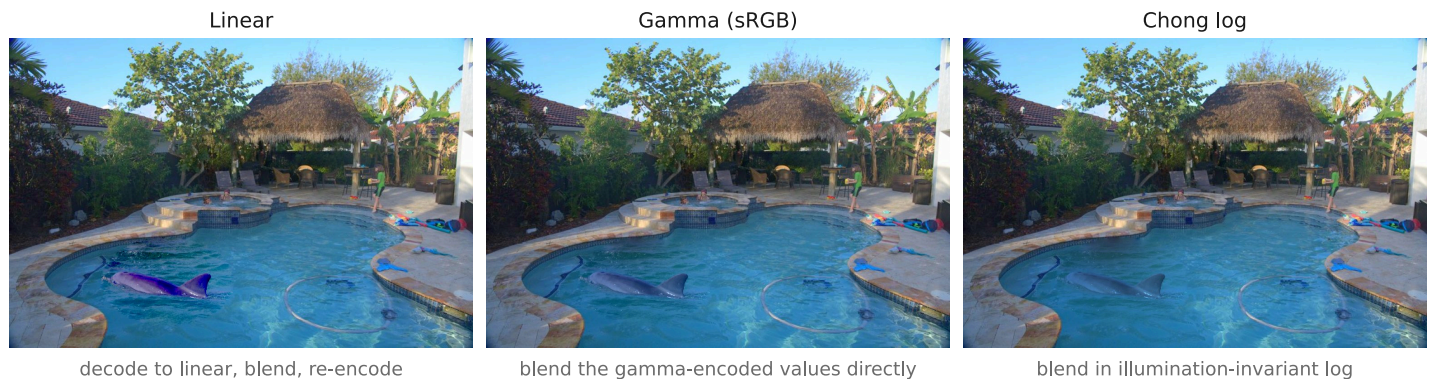
Figure 8.2.1 ( reproduced ). The same seamless clone, solved in three color encodings. One composite (a dolphin cloned into a pool) run through the identical Poisson solve in linear, gamma, and Chong's illumination-invariant log space ( Chong et al. 2008 ), then converted back to sRGB for display, so the only difference between the panels is the space the arithmetic ran in. The re-leveling that hides the seam behaves differently in each: linear leaves the pasted dolphin a garish purple, gamma is milder, and log lands closest to a natural gray. A forward reference; the interactive version and the full story are in Chapter 10.8, Poisson image editing .
